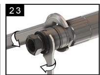
If you experience loosening of threaded joints during shooting it is recommended to degrease the threads and use a quality thread locker such as Vibra-Tite 123.
