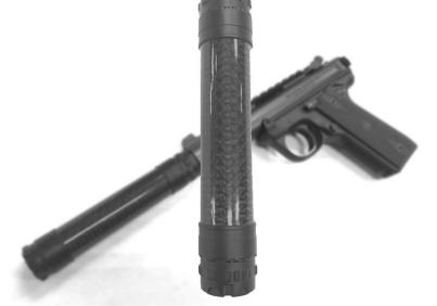
Prior to use, ensure all threaded junctions are properly shouldered against their corresponding surfaces and tightly secured. For ease of cleaning, consider lightly coating the interior surfaces baffles in a viscous oil/lubricant prior to use to limit the sticking of carbon and other debris. Never coat the exterior of the baffles that are in contact with the carbon fiber tube.
